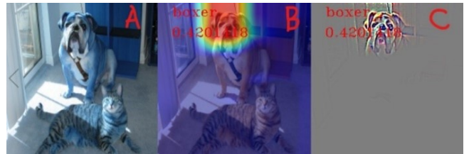
Figure 5: Visualize VGG16 network using CAM and GBP methods. (A) Original image. (B) Class Activation Mapping. (C) Guided-Backpropagation. [7]
